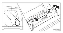
Holding the green inset grips of the new photoconductor unit, insert the unit into the photoconductor unit holder.
